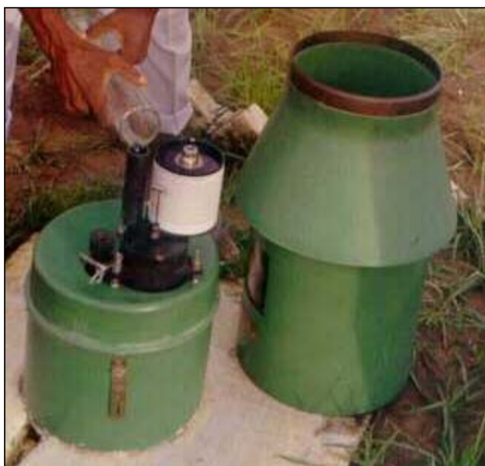
Figure 6.2: Autographic natural siphon rain gauge (ARG)
