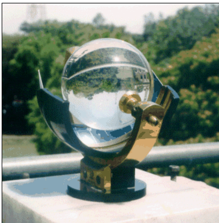
Figure 6.5: Campbell-Stokes sunshine recorder (Latitude 5°S to 45°N)
