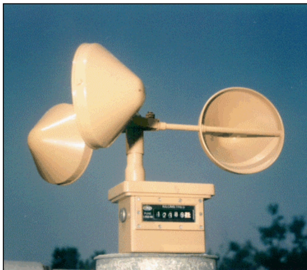
Figure 6.12: General arrangement of cup counter anemometer
